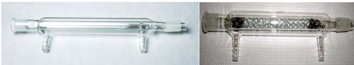
Distilling Column (Fractionation Column – without and with fractionating material, glass beads, inside)
